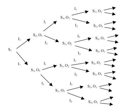
Figure 1: Contingency tree for the coke machine FSA
